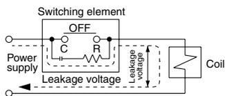
Keep the residual leakage voltage with 2% of the rated voltage.
