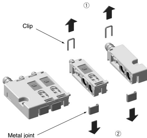
To remove the station, follow the same procedure for assembly and disassembly.
