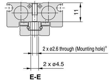
\* Use the attached hexagon socket head screws for mounting holes.
