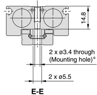
\* Use the attached hexagon socket head screws for mounting holes.
