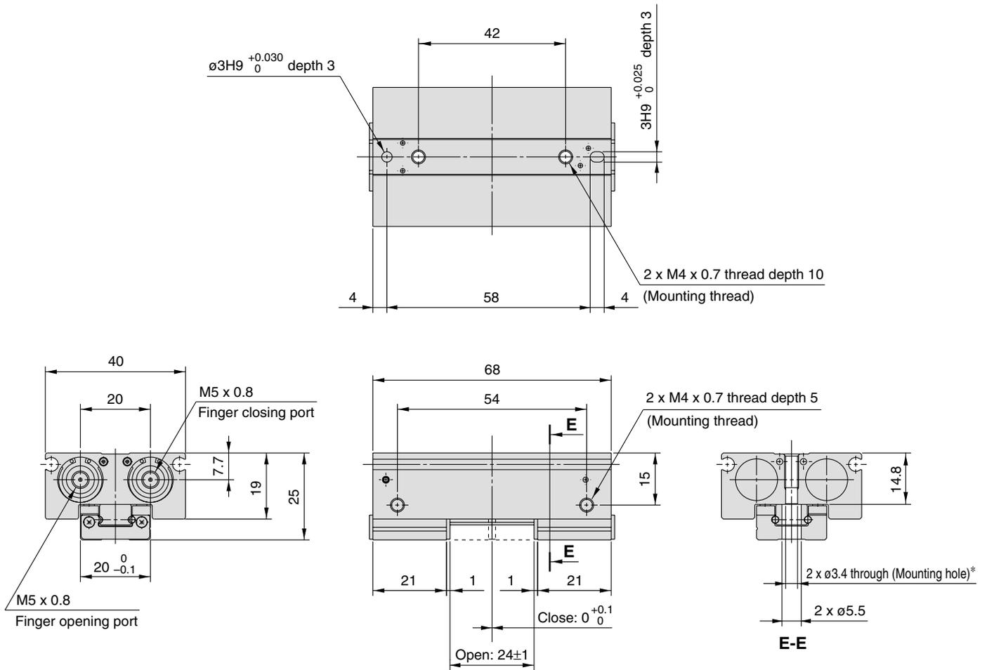
\* Use the attached hexagon socket head screws for mounting holes.
