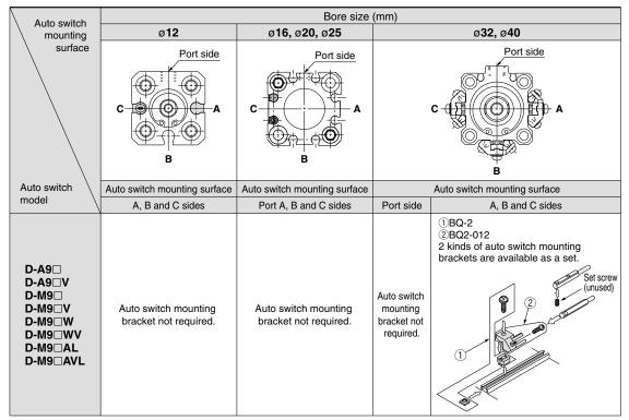
Note 1) For each cylinder series, when a compact auto switch is mounted on the three sides (A, B and C above) other than the port side of bore sizes ø32 and ø40, the auto switch mounting brackets above are required. Order them separately from cylinders. Order example
