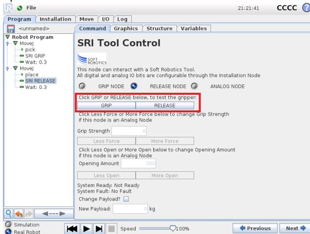
If the “Change Payload?” checkbox is CHECKED, the value in the “New Payload” field will be set as the current robot payload. This is the total mass of the EOAT and the Payload.
