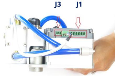
1. Install cable harnesses into SRCU-Mini UR+ controller. "J3" is the power cable, and "J1" is IO. See Section 1E: Product Overview for additional depiction of the SRCU-Mini UR+.
