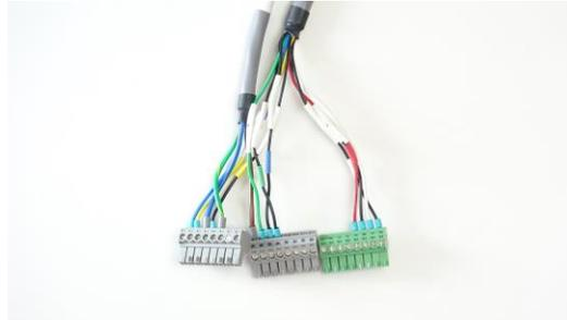
1. Remove Universal Robot Controller Terminals “Analog”, “Digital Inputs” and “Digital Outputs”, that correspond with below wiring diagram, from the Universal Robot Controller.
