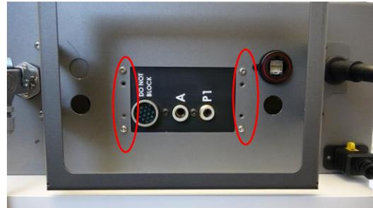
4. Re-use the UR Controller Cabinet access panel screws to mount the SRCU-Mini UR+ to the cabinet. Please note, depending on your Universal Robot series, your access panel may have (8) or (6) holes.
