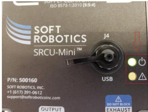
1. Power on system by pressing power button on Universal Robot teach pendant. The SRCU-Mini UR+ will only power up once the teach pendant has completed booting and entered the home screen.
