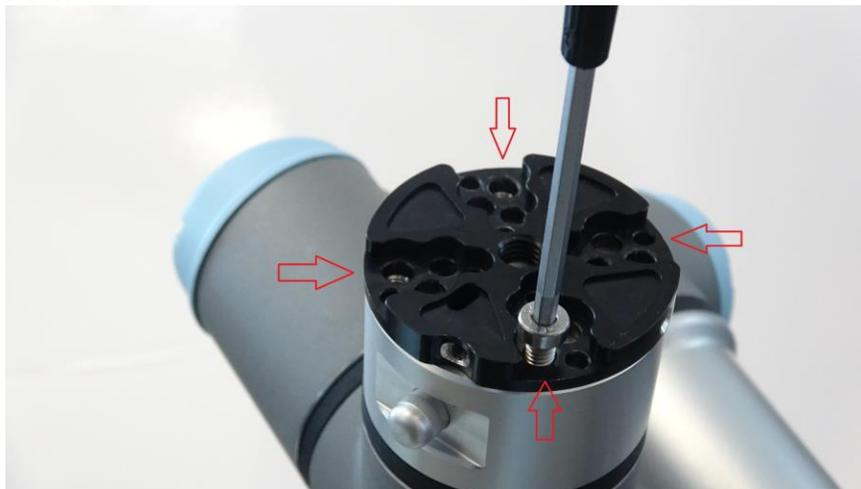
2. Mount preconfigured SRDK EOAT to robot side Universal Mounting Plate using (4) M4x16 socket head cap screws and aligning key way. Use the 2.5mm hex screwdriver for mounting.
