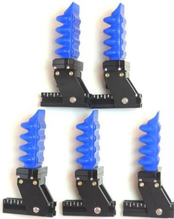
Whether the shape of the product resembles a square, circle, rectangle, or ellipse will change the number of Finger Modules required for the application. If a product has more of a square or circular form factor an EOAT with between 2 and 5 Finger Modules would be most effective. Where a product that has more of a rectangular or elliptical form factor would require between 4 and 6 Finger Modules.
