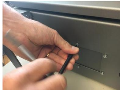
2. Remove bottom access panel from UR Controller using T20 Torx Driver
