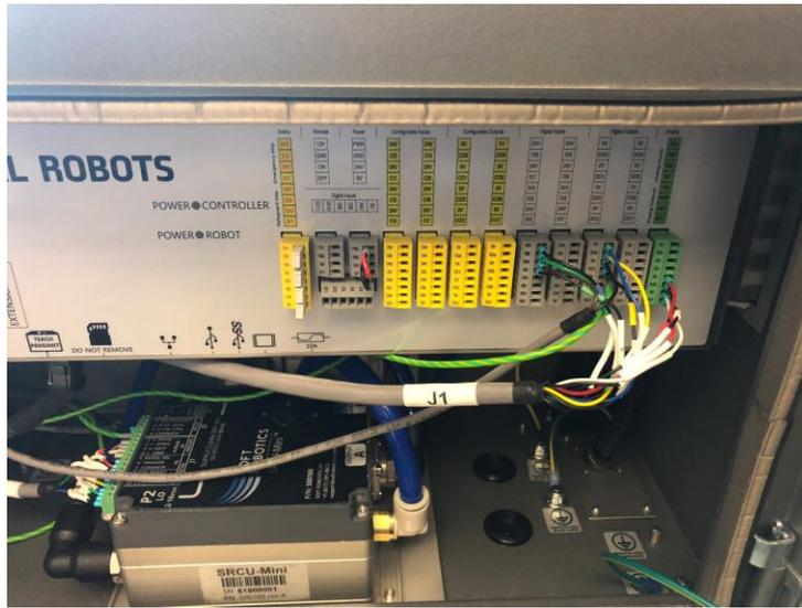
3. Reconnect terminal strips to appropriate locations on Universal Robot Controller.
