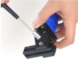
2. To adjust the position of the finger module on the rail, use your 7mm nut driver or hex wrench (depending on accessibility) to slightly loosen rail screw on either side of rail. Slide forwards or backwards to needed position. Once repositioned, tighten rail screws.
