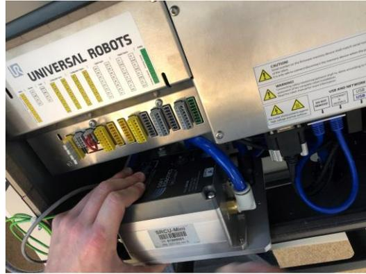
3. Carefully insert the SRCU-Mini UR+ so as to not damage pneumatic fittings or any electrical connectors. Orientation for insertion is referenced in above photos.
