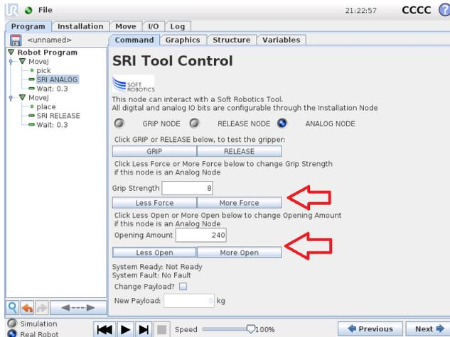
You can manually actuate your SRDK-UR+ EOAT using the **GRIP** and **RELEASE** buttons as shown below. This is for real time testing of grip and release functionality. The radio buttons, i.e. “GRIP NODE”, control the runtime operation of the node.
