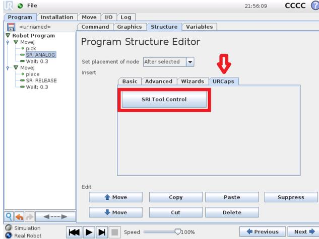
8. There are (3) different options for controlling the SRDK EOAT. **Grip** is used to pick an object. **Release** is used when placing an object. **Analog** is used to change your **Grip Strength** and/or **Opening Amount** prior to reselecting **Grip Node** or **Release Node**.
