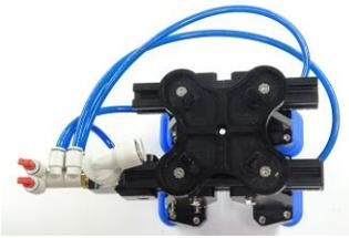
When connecting the Pneumatic Manifold to the Pneumatic Module the appropriate air tubing length should be considered. The orientation of any air tubing should not interfere with the actuation of the EOAT. Similar length air tubing should be used to feed the Finger Modules from the Pneumatic Manifold. This will assure actuation symmetry.
