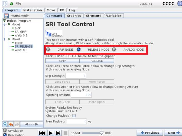
When “ANALOG NODE” is selected, “Grip Strength” and “Opening Amount” can be adjusted. Valid values for **Grip Strength** are **0** and **2 to 14**. Valid values for **Opening Amount** are **0 to 480**.
