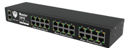
Master 2410. Supports up to 24 sensors.
