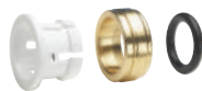
WHITE ACETAL COLLET ON 1/4" BLACK ACETAL COLLET ON 5/32" GRAY ACETAL COLLET ON 3/8" AND 5/8" BRASS BODY EPDM O-ring
