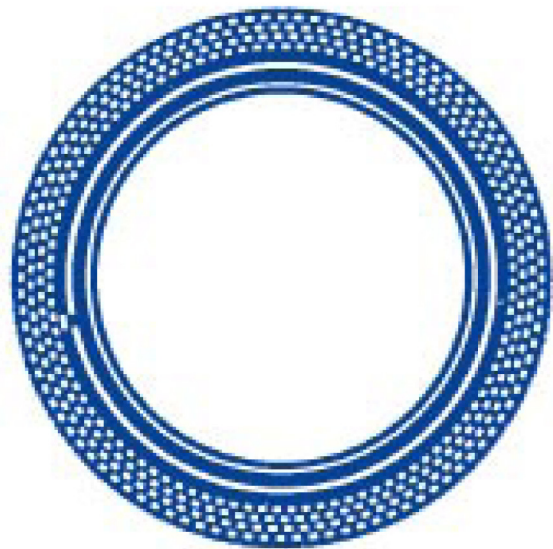
Figure 2: Code disc for an optical quadrature encoder shows the inner ring for the Z channel, which generates a single pulse per revolution. The outer bands correspond to the A channel and B channel; notice that they are offset by 90°.
