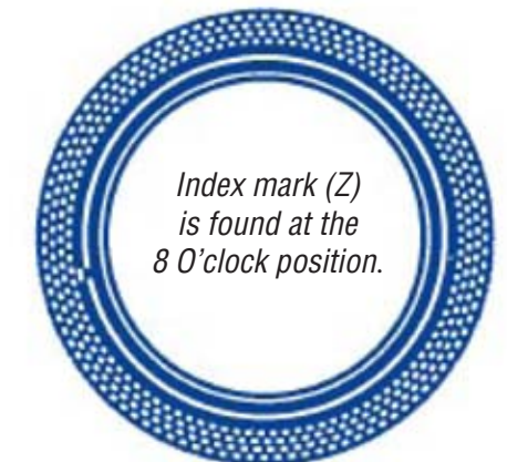
Figure 3: Code disc for an optical quadrature encoder shows the inner ring for the Z channel, which generates a single pulse per revolution. The outer bands correspond to the A channel and B channel; notice that they are offset by 90°.
