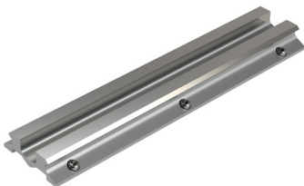
Track plate assembly consisting of two or more lengths of induction hardened steel track mounted to an anodized aluminum substrate
