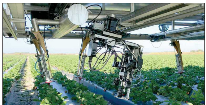
In precision agriculture, this high-speed automated picker uses corrosion-resistant LoPro actuators to work consecutive 20 hour days in all weather conditions and heavy debris.
